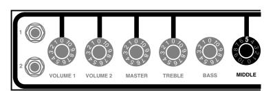
need midrange for punch and attack to produce a bigger, bolder sound. An interesting sound in channel 1 for lead playing is achieved by turning the TREBLE and BASS Controls to 0, and the MIDDLE Control to 10. This will reveal the frequencies that this control works with, as well as producing a fat, warm and very smooth tone.
